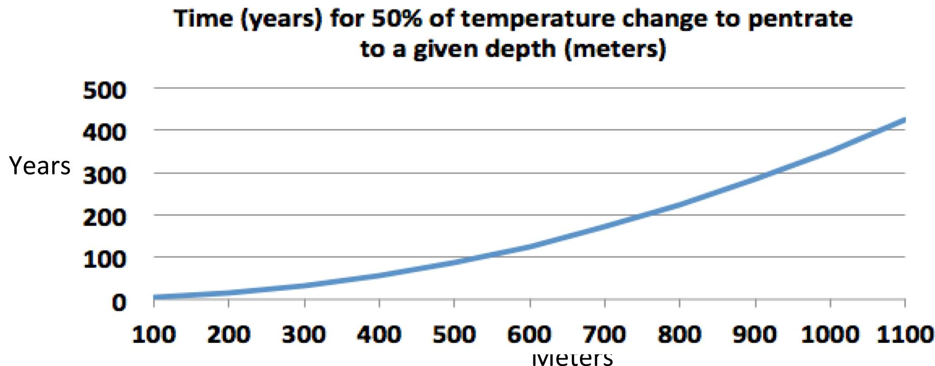
The above graph exaggerates the rate of heat penetration into the ocean because the general ocean uplift slows down the downward diffusion of heat. The depictions of the ocean shown above are idealized. At times and places the mixed layer may almost disappear or conversely become several hundred meters deep. In polar regions the stratification of the ocean often disappears entirely with uniform temperature reaching to the bottom.
