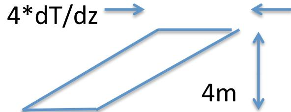
Heat added per year per cubic meter if uplift was working alone  $4.18 \times 10^6 \cdot dT/dz$  joules.  $dT/dz \sim 0.1$  tropical thermocline. Differential flux in watts for a cubic meter:  $\sim .013$  watts/sq m stays in cubic meter volume
