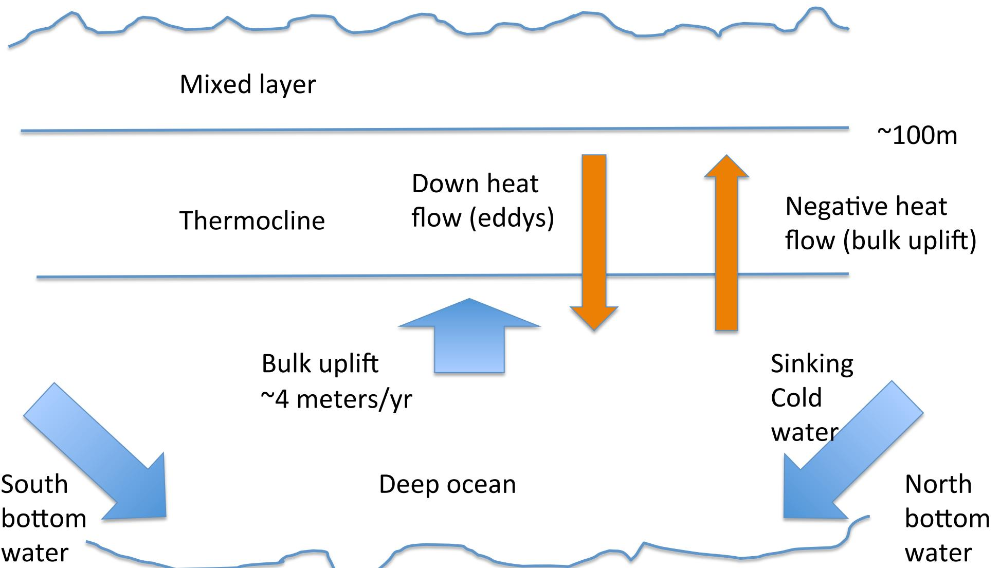
For a steady state net heat flow at any level is zero – downward flow of heat from warm to cold is balanced by bulk uplift of cold water.
