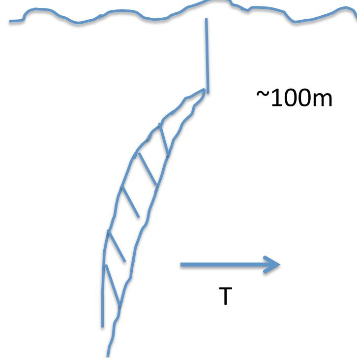
How long does it take for heat to penetrate down in the ocean? The analytical Solution for step function input to the 1-dimensional heat equation gives a rough answer.
